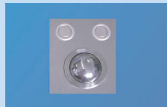
Stainless steel trackball 38mm with 2 buttons
